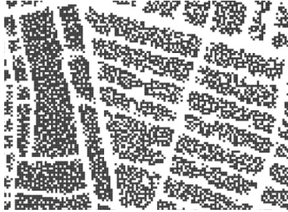
Figure 6. An image depicting the developed simulation environment utilising smaller sub-grids separated by a perpetually 'dead' street cell.
